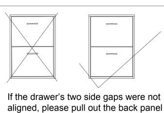
If the drawer's two side gaps were not aligned, please pull out the back panel nails and adjust the cabinet angles to ensure the frame angles are square. After the drawers are fully aligned and travel smoothly, fully hammer nails to inside back panel.
